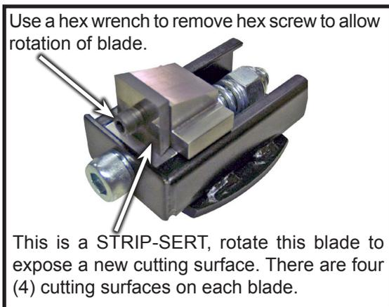
**STRIP-Serts™** Are carbide-tipped blocks designed to clean floors without grinding into the concrete. The multi-sided, replaceable tungsten carbides have four edges that can be rotated for maximum use. The carbide Strip-Serts™ will clean your surface without any damage.
