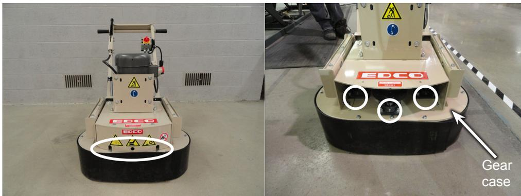
To grease the flange bearings attach the grease gun to the grease fittings through the access holes circled in photo above left and give only two (2) pumps on the grease gun every 50 hours of use. If excessive over lubrication is done grease will leak onto the work surface causing possible damage and wasted cleanup time. Inspection hole on gear case is located towards rear center of machine on top of gear case.
