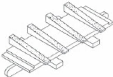
The above is an example of a DYMA-SERT that has not been rotated after every four hours of use. To get maximum life out of a DYMA-SERT they should be rotated 180° every four hours of use.
