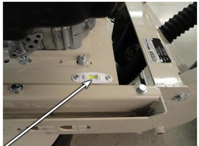
Rock the machine back and forth until the bubble level is centered.
