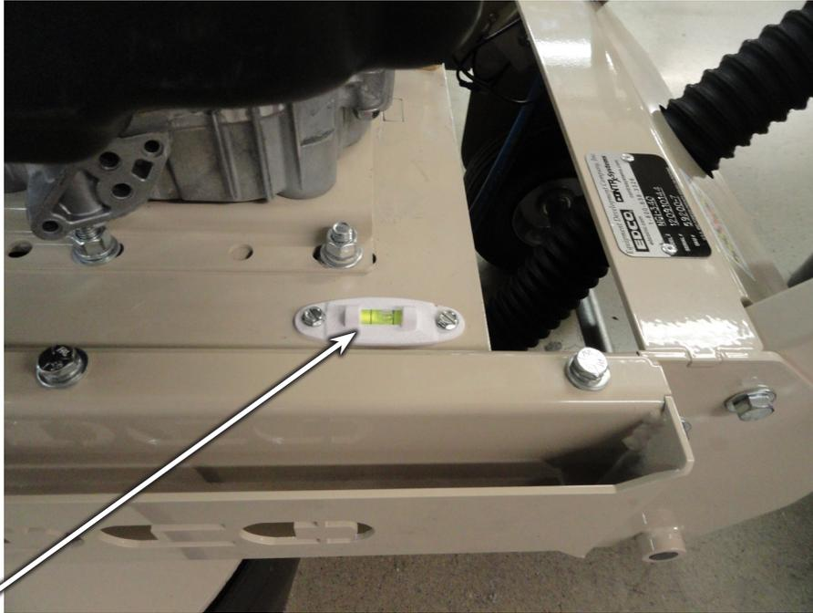
The bubble on the machine will not necessarily be centered once optimum operating position is achieved. It will also float back and forth during grinding. Level on your machine may not be the same as pictured above.
