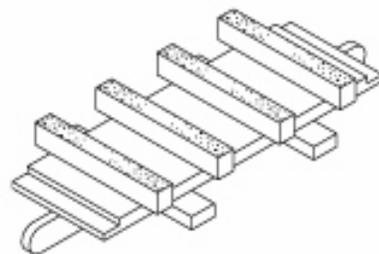
The above is an example of a DYMA-SERT that has been rotated after every four hours of use, as you can see the wear is even across all segments.
